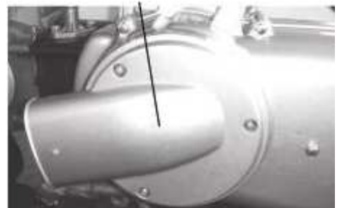
Left crank shaft cover air inlet
