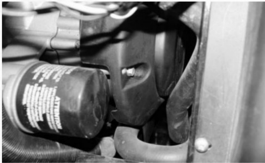
1. Engine oil drain bolt
