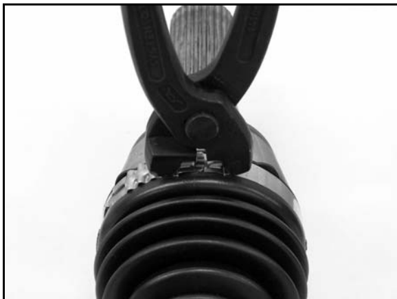
Axle Boot Clamp Tool PU-48951
