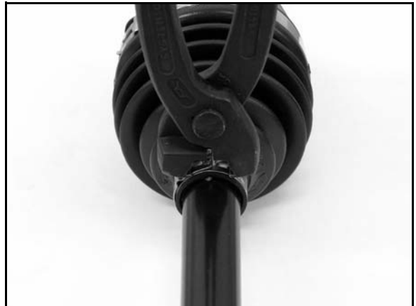
Axle Boot Clamp Tool PU-48951
