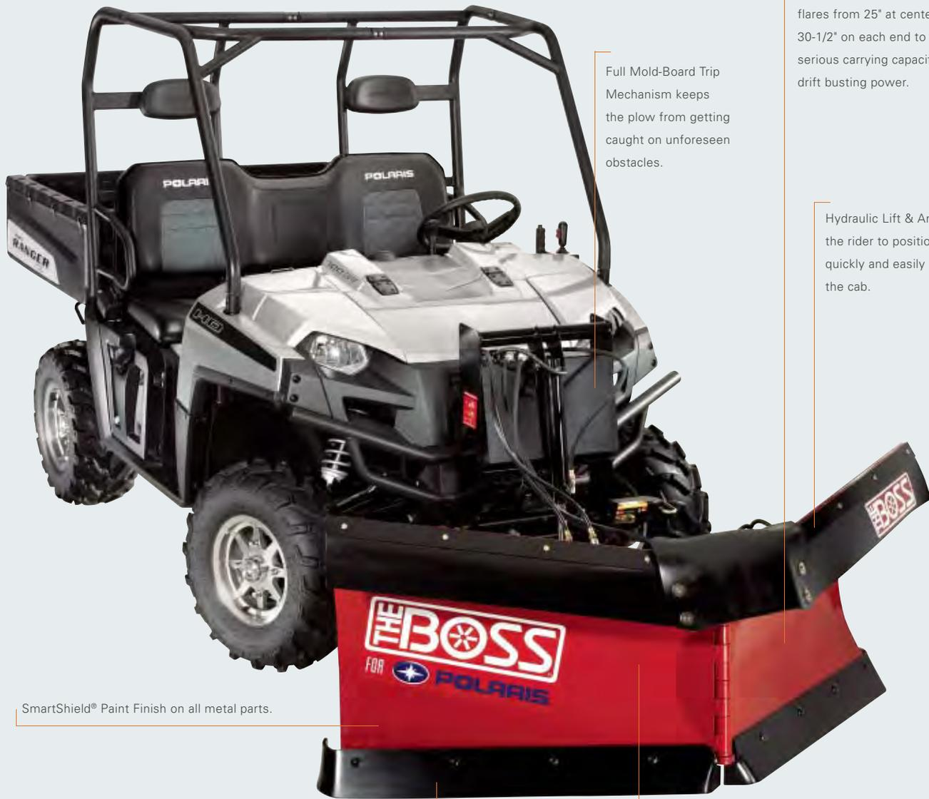
Full Mold-Board Trip Mechanism keeps the plow from getting caught on unforeseen obstacles.
