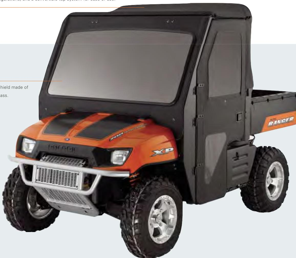
Fixed glass windshield made of laminate safety glass.
