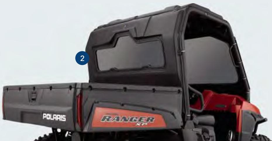
\*Adding a windshield to any open air vehicle causes a low pressure area behind the windshield that attracts dust to this area. To minimize this effect, Polaris recommends the use of the Pure Polaris Rear Panel any time a windshield is installed.
