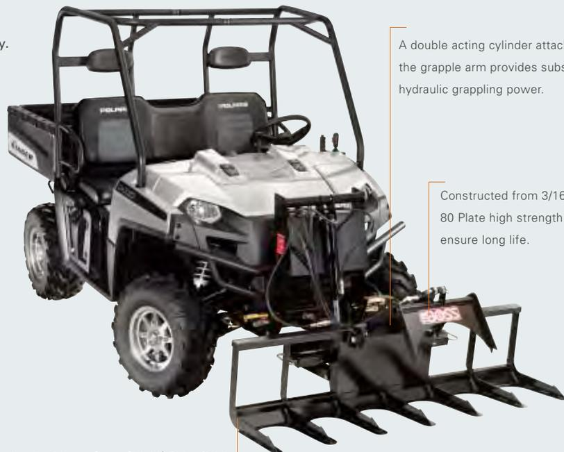
A double acting cylinder attached to the grapple arm provides substantial hydraulic grappling power.
