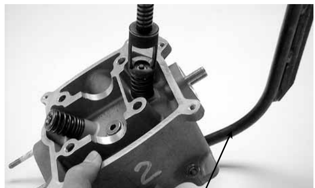
Valve Spring Compressor
