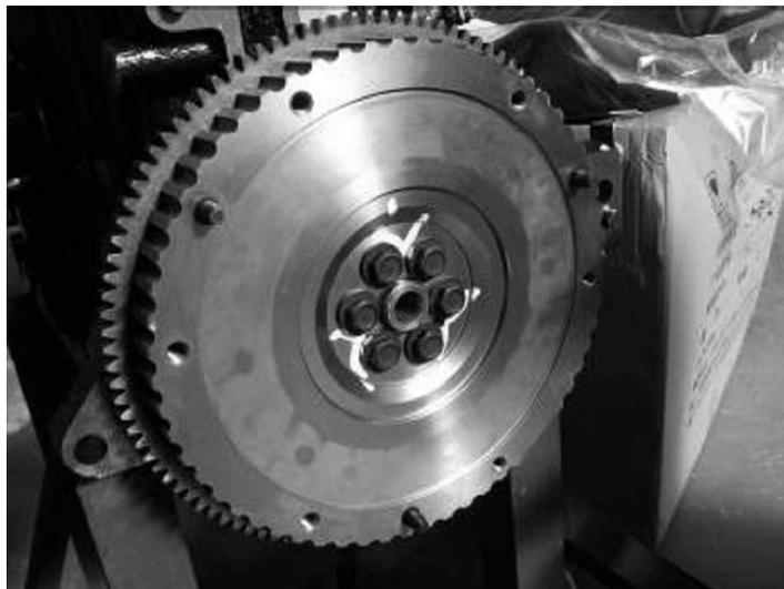
5. Insert a spline-shaft into the hole of the Clutch assy , fix the six bolts on the Clutch pressure plate ,tighten them according to the prescribed torque 28 N.M .
