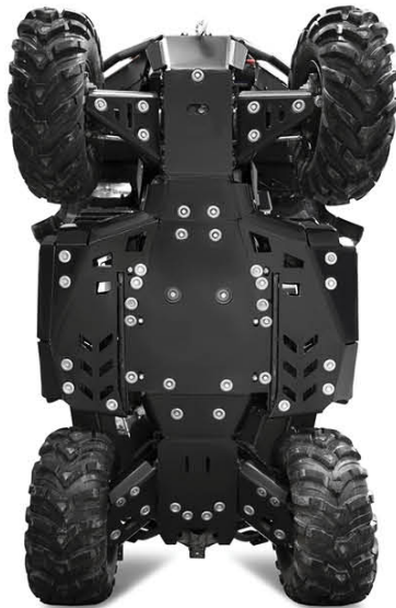
Plastic skid plate kit for CF MOTO CFORCE 600/625 Touring (8 mm) K.8103.1
