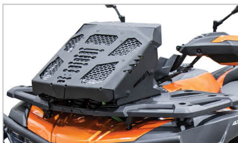
Radiator relocation kit with snorkels CFMOTO CFORCE 600/625 (2020-) / X5 H.O. (2015-) + fitting kit 2444.8114.1
