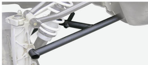
Suspension arms kit for Arctic Cat Bearcat 570XT/ 570XTE/ Z1 XT/ 2000 XT/ 2000 XTE/ 5000 XT 5.7302.1
