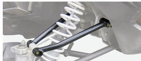
Suspension arms kit for Arctic Cat Bearcat 570XT/ 570XTE/ Z1 XT/ 2000 XT/ 2000 XTE/ 5000 XT 5.7301.1
