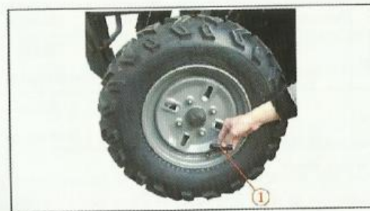
① Inductive tachometer
