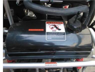
Fuel tank capacity = 9 Litres or 2.5 gallon
