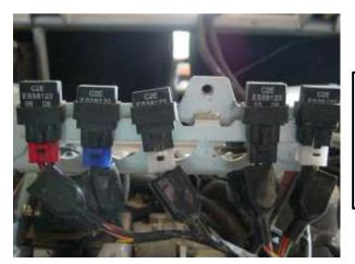
Red: main relay Blue: high beam relay White: low beam relay Black: cooling fan relay White: fuel pump relay
