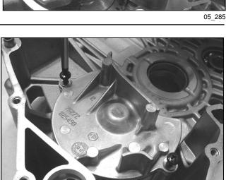
**Tightening torque** Gate fixing screws: 8 - 10 N·m
