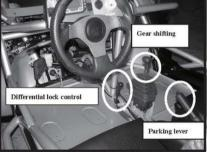
4. <u>Gear shifting:</u> Refer to the gear shift box as below photo, practice making gear lever slide into correct position. Be more familiar with the gear lever shift route, and it will get easier to enjoy driving.
