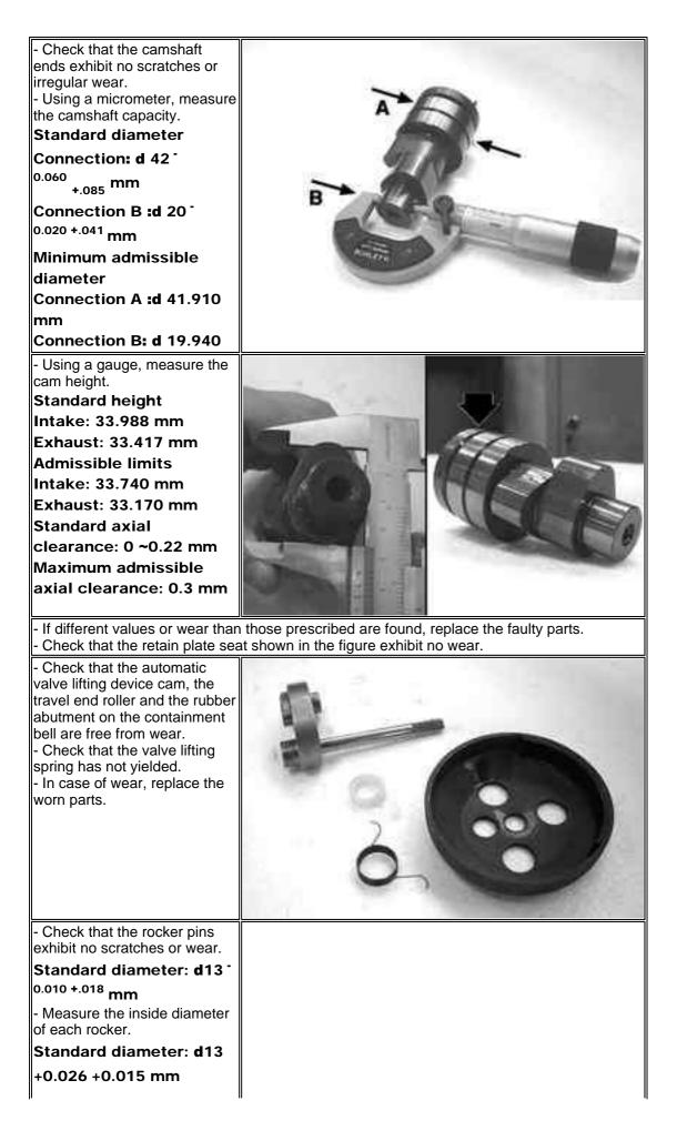
Check that the cam contact sliding block and the articulated register plate is free from wear.
