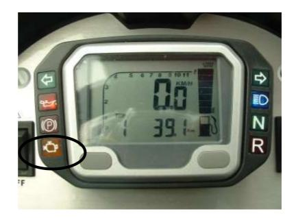
Failures are detected and restored by the diagnostic tester dwg. 020460Y. In any case, when the fault has been fixed the stored value is automatically deleted after 16 usage cycles (cold start, running in temperature, stop). The diagnostic tester is also
