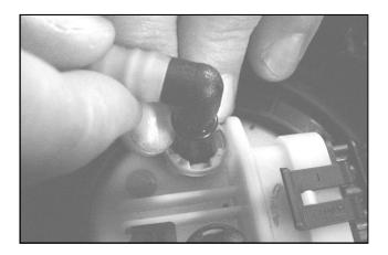
System pressure control, for practical reasons, must be carried out by connecting to the pump side.
