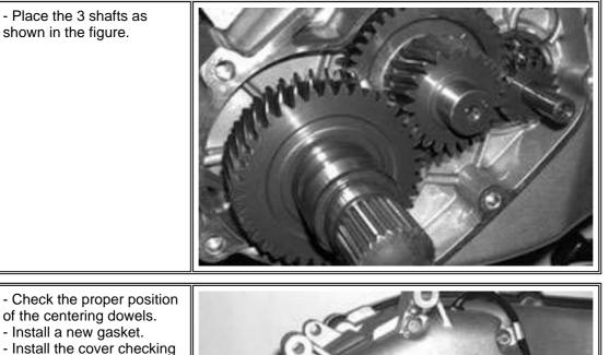
of the centering dowels. - Install a new gasket. - Install the cover checking
