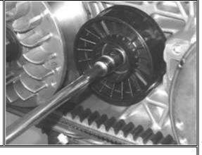
Tightening torque: Anti-flapping roller screw: 16,7 ~19,6 Nm Prepare the specific tool as for removal;
