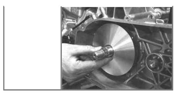
Install the belt anti-flapping roller with the containment edge on the engine crankcase side.
