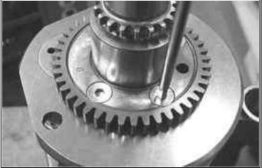
Blow with compressed air and degrease the fixingholes on both surfaces to make the new LOCTITE grip. Apply LOCTITE 243 to the holes again.
