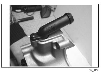
Tightening torque: Blow-by recovery duct fixing screws: 3 - 4 N·m
