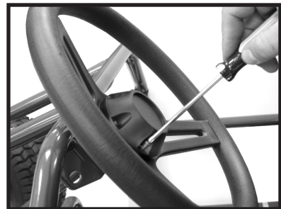
Attach with Phillips head screw (A).
