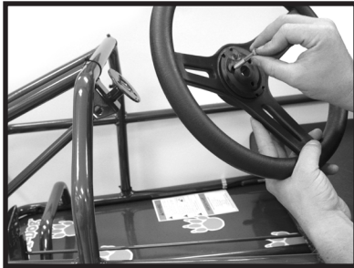
Slide 1/4" Hex Bolts (9) through holes in steering wheel.
