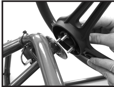
Insert Assembly through holes of steering shaft.
