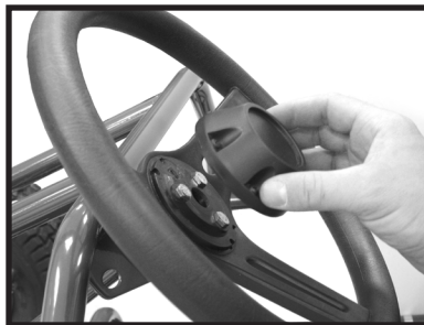
Place steering wheel cap over center of steering wheel.
