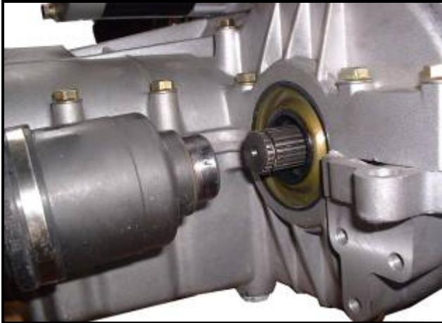
1. **Caution: the Steel cable baffle ring-3 must be confirmed in the groove both sides before attaching drive shaft.**
