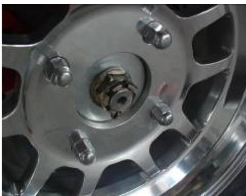
1. Attach wheel (27X11-12),BR-2 on the hub. tighten the nuts-3.
