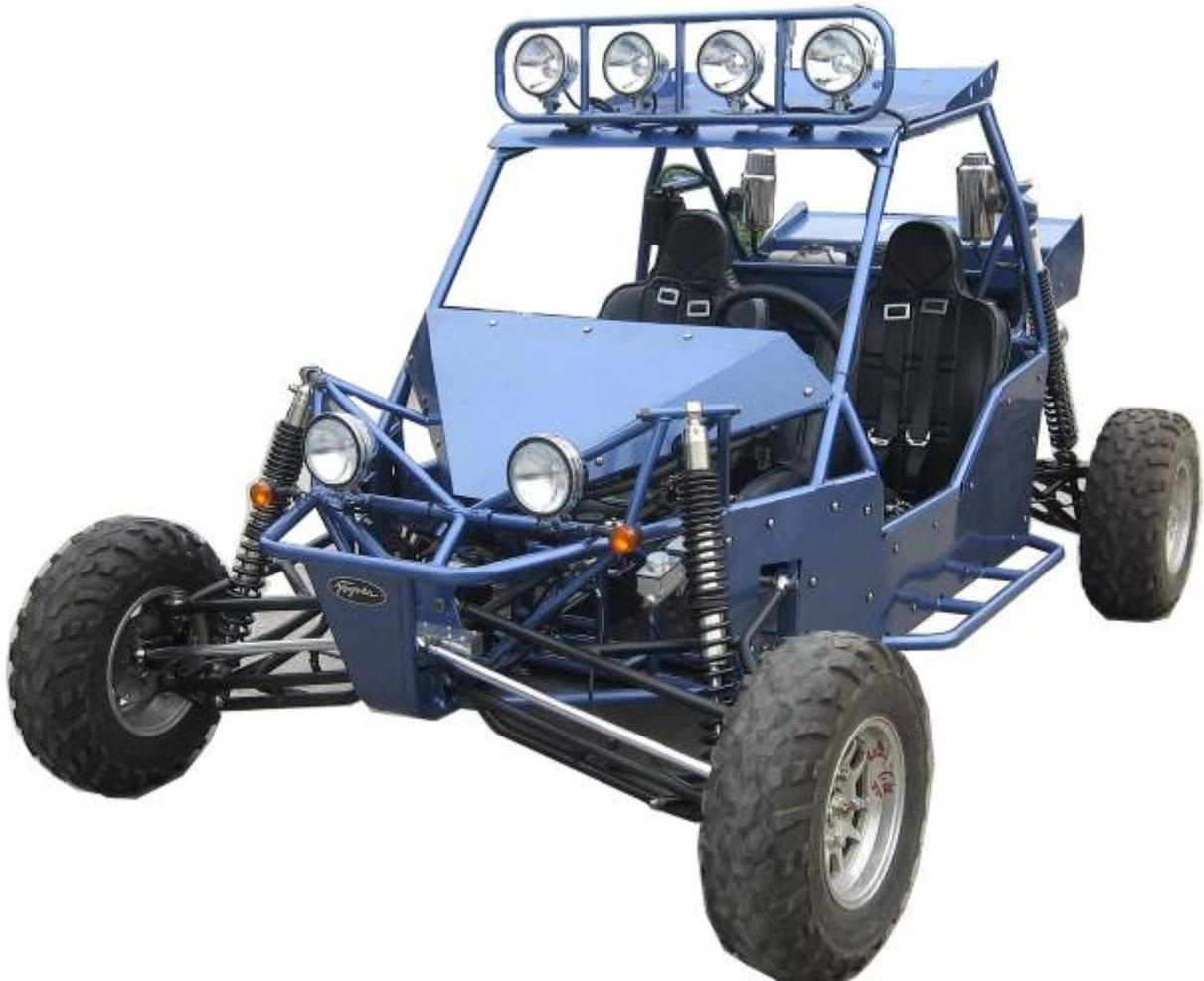
1. Before starting the engine check engine oil, gearbox oil and all plugs have good connection. check the level of coolant at the filler neck of inlet to radiator after leaving the cap off at this stage. check pressure in the tire; front tire: 15psi; rear tire: 15psi check all bolts and nuts are tight.
