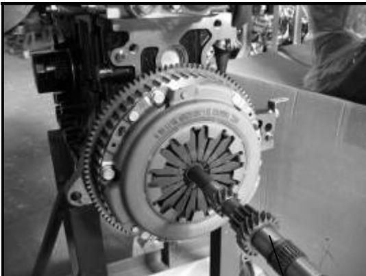
**FIGURE 27** Spline-shaft
