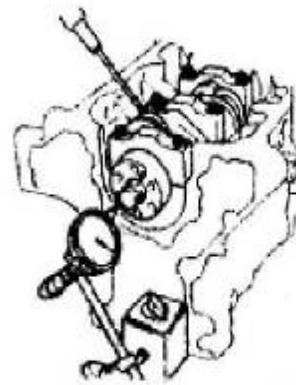
2.3. Use a caliper to measure the crankshaft axial
