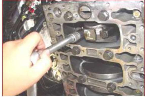
6) Remove the connecting rod bearing lower cover.
