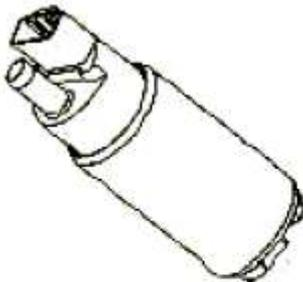
Chart 3-12 Exterior Drawing of Electric Fuel Pump
