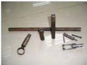
SST for valve oil seal
