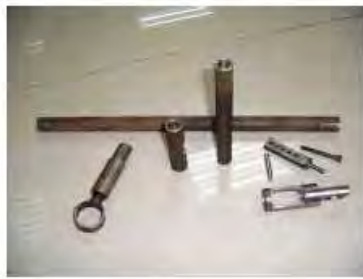
SST for valve oil seal
